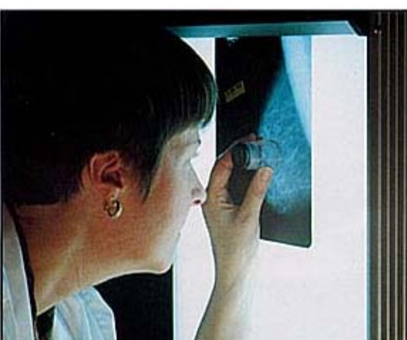
Use a viewbox and eye loupe with at least 7x magnification to inspect any artifacts on the film.
